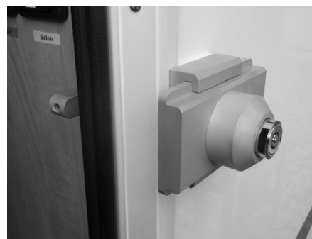
10 – Fit handle and secure firmly in position (top of lock open)
